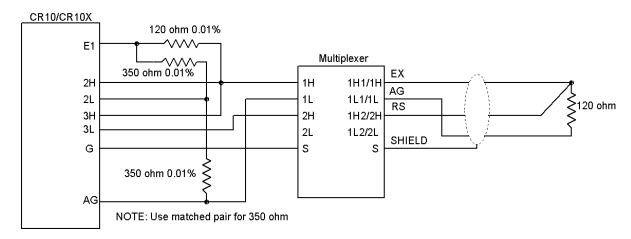
Contact Canary Systems to obtain the required precision resistors. It is essential to use high accuracy low-temperature coefficient fixed resistors.
