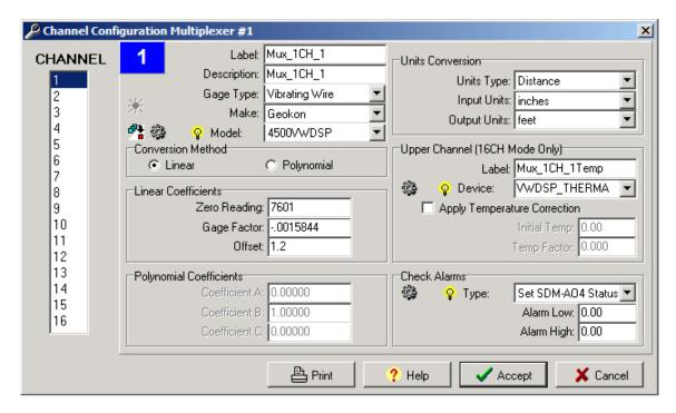
Note: The Zero Reading must be obtained in the field. It is recommended to run the Zero function to obtain these results. Enter the (negative) Gage Factor in inches or millimeters per digit from the 4675LV Calibration Sheet. Measure the depth of water at the time of the Zero Reading and enter this value as the Offset shown above, it must be the same units as the Units Conversion selection.
